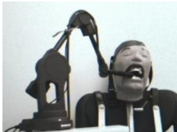
Fig. 3. The experimental setup of the proposed system consists of a CCD camera mounted on a five link 3D digitizer. A DC regulated light source is connected to a fiber optic bundle surrounding the camera. The setup is connected to an SGI Indigo2 machine.
